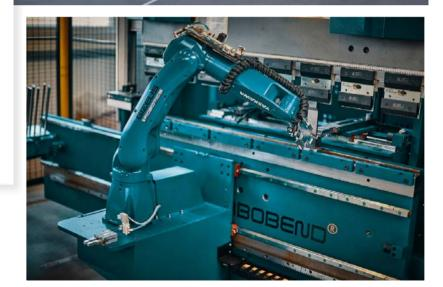
"RoboBend is a truly flexible system. When the amount of pieces is large, we feed the robot, and that works for us. When the amount is small or we want to test a new product, we operate the press brake manually. In this case the robot remains in an Emergency Stop state at the parking spot, allowing us to use the entire length of the press brake machine." the operators say.
