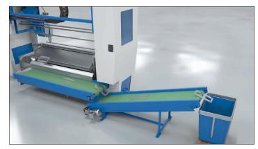
Additional conveyor to unloading point
