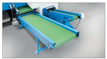
Double conveyor to unloading point
